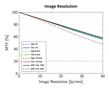
Modulation Transfer Function (MTF) vs. Image Resolution, wavelength range 486 nm - 656 nm. Fields in legend are represented as distance from the center of the boroscope tip
